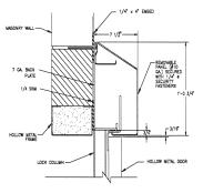
**COVER BOX SECTION** 7-1/8" deep x 1' - 0-3/4" tall cover box field welded 1" on 8" ton and hottom.
