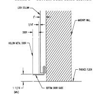
Flush receiver jamb allows frame opening and clear opening to he the same
