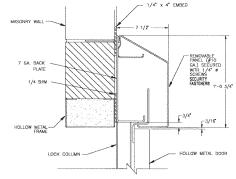
**COVER BOX SECTION** 7-1/2" deep x 1'-0-3/4" tall cover box field welded 1" on 6" top and bottom
