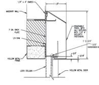
**COVER BOX SECTION** 7-1/2" deep x 1' - 0-3/4" tall cover box field welded 1" on 8" top and bottom.
