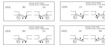
\* Indicates lock mounting/access plate side.
