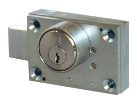
The key cannot be removed from the lock unless the bolt is fully extended (i.e. deadlocked) or fully retracted. This safety feature alerts the user to an obstruction in the bolt keeper or receiver which might jeopardize security.
